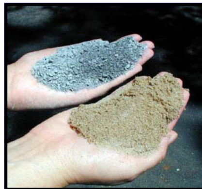
Note the difference in the size of the sand. The smaller particle sized, light tan colored sand is used for a sand filter.
