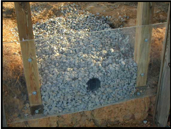
Conventional gravel trench with 4" inch perforated pipe.
