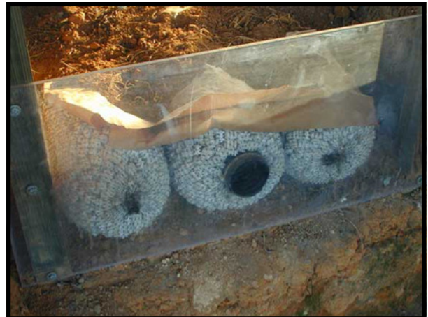
Perforated flexible 4" inch pipe (Expanded Polystyrene Bundles).
